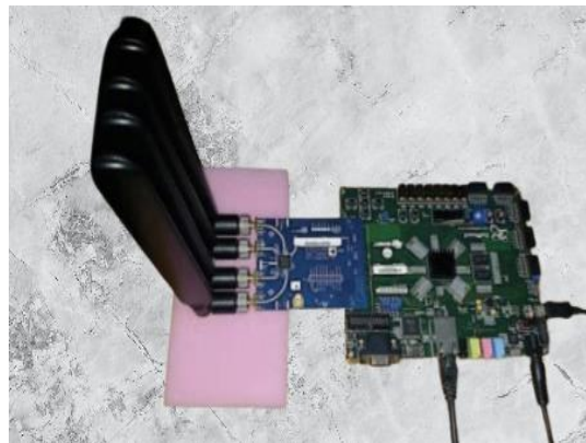
Fig.4 Interfacing of AD9361 With FPGA
